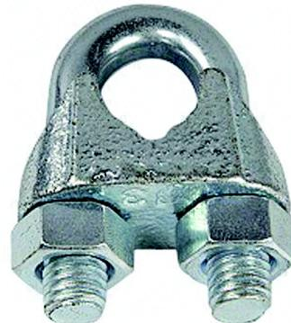
Malleable Wire Rope Clips. These clips are intended for use in making eye termination in right regular lay wire rope. Such an assembly is for non-critical light duty use where a small applied load is expected such as hand rails, fencing, guard lines, etc. For this reason an efficiency of the termination is not stated.
