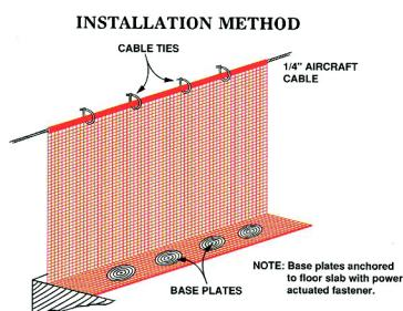
OSHA 1926.500-Subpart M requires guardrail and toeboard systems on all open-sided floors, platforms, runways, wall openings, holes, roofs, excavations, and machinery areas. Additionally, when equipment or materials are piled higher than the top edge of a standard toeboard, debris netting must be installed from the top rail to deck level to provide overhead protection for employees working below.
